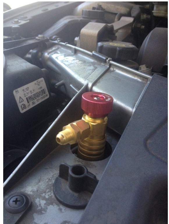
New coupler shown fitted to the concealed high side charge port of a 2008 MA Ford Mondeo
