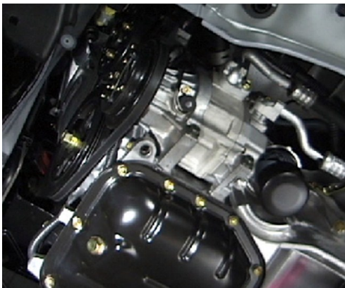
2001-2003 GENERATION 1 TOYOTA PRIUS BELT DRIVEN COMPRESSOR.
