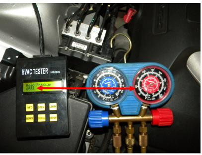
Connect a high side pressure gauge set and the VE HVAC scan tool. Start the vehicle and engage the A/C. At idle compare the scan tool value to the actual high side pressure they should be approximately the same values. (+/- 5%)
