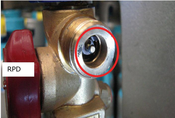
Empty returned charging cylinders (white or with light blue band) must have the RPD (residual pressure device) fitted.
