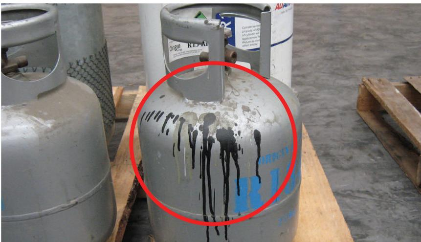
No paint, texta pen marks are to be on the cylinders. All cylinders are supplied with a tag affixed. Any information can be provided on that tag.
